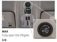
Open the liftgate to the programmed height.
